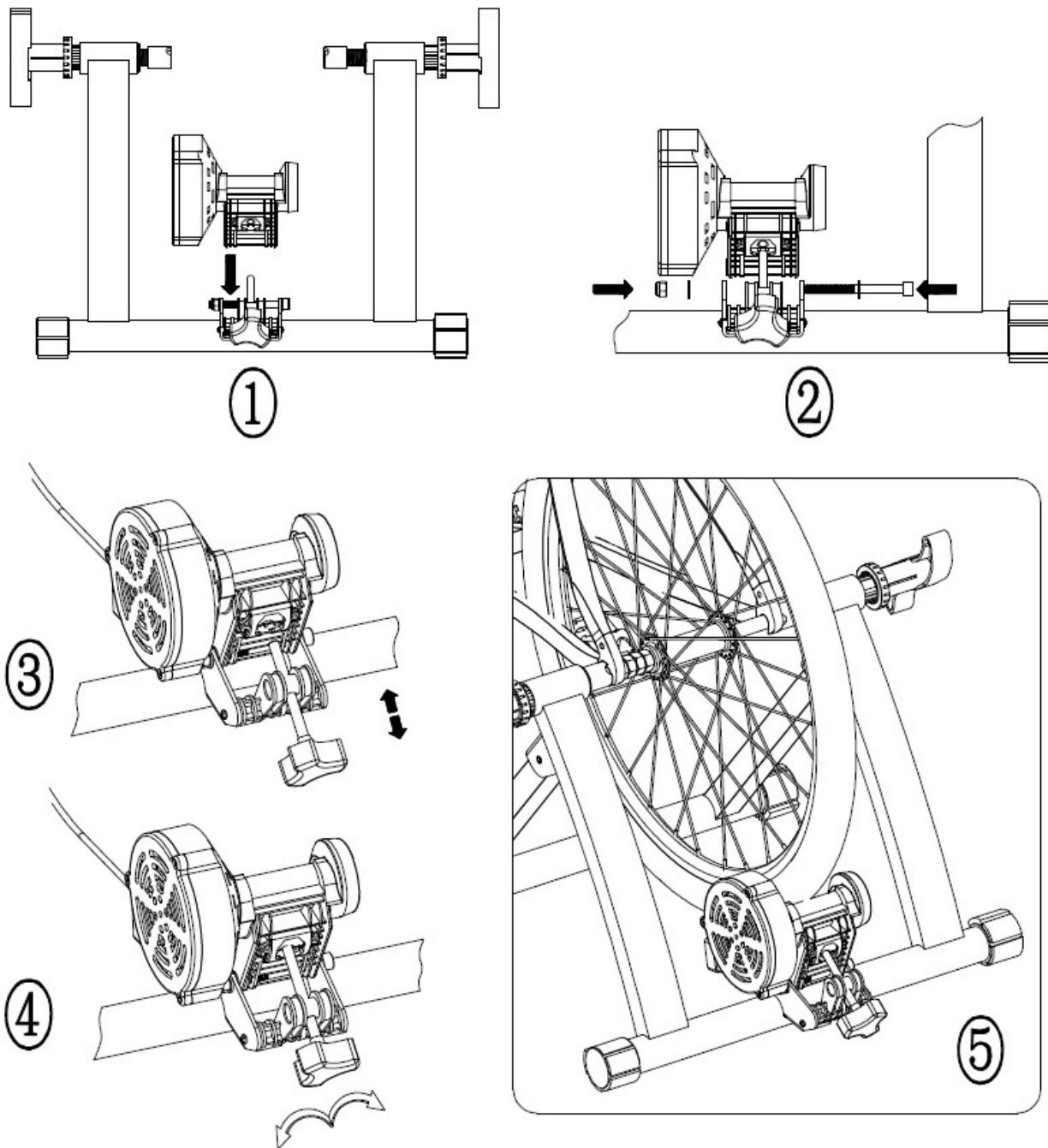
6. Install the control clamp on the handle bar and tighten handlebar nut securely.
